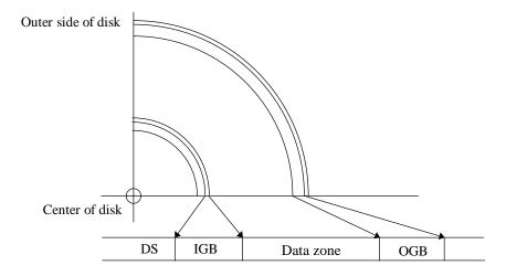
Figure 8.5 Position of servo track
